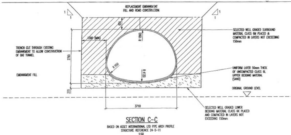
Figure 2. Bat culvert in section.
