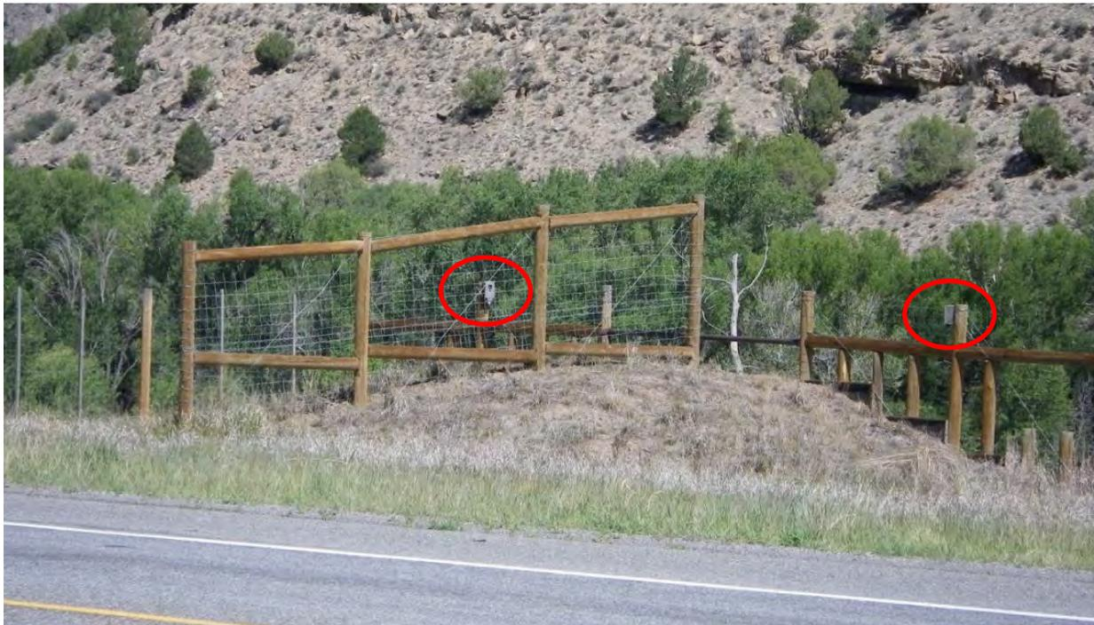
**FIGURE 2** A representative escape ramp along Highway 550 depicting camera placement (cameras circled in red).
