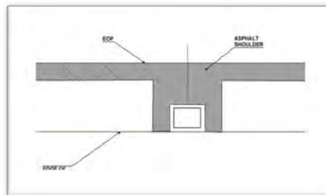
**FIGURE 8 Ditch Bottom Inlet Plan View**
