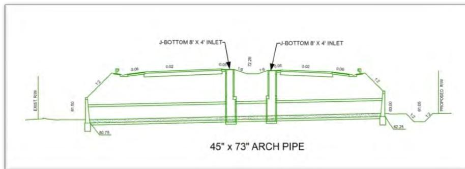
**FIGURE 7 Arch Pipe Showing Ditch Bottom Inlets**
