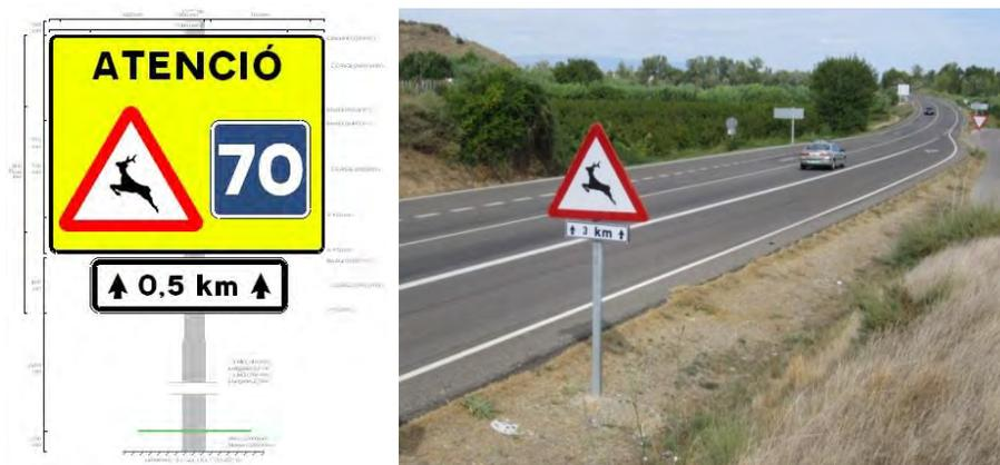
**Figure 7. Specific additional signalization, installed during the critical period (September to January) at ungulate-vehicle collision hotspots that are qualified as a ‘priority’ (left). Along other conflictive stretches, standard warning signs (right) are installed.**
