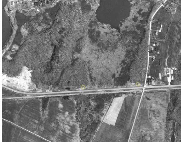
Fig. 3. Aerial view of the segment planned for installation of box culverts and land conservation. The yellow points indicate the proposed locations for box culvert placement.
