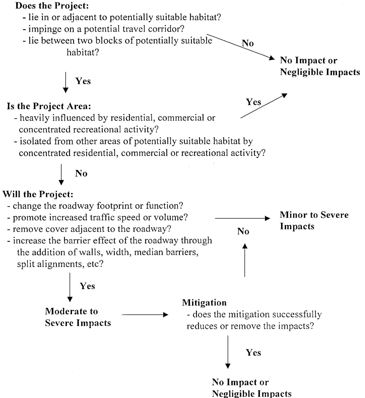
**Figure 3.** The process for determining initial project impacts. e.g., the level of impact that will occur before mitigation. The questions posed in the flow chart are answered based on the background material presented in Chapter 3, project specific information, and the best available information about the status and habitat use of lynx in Colorado
