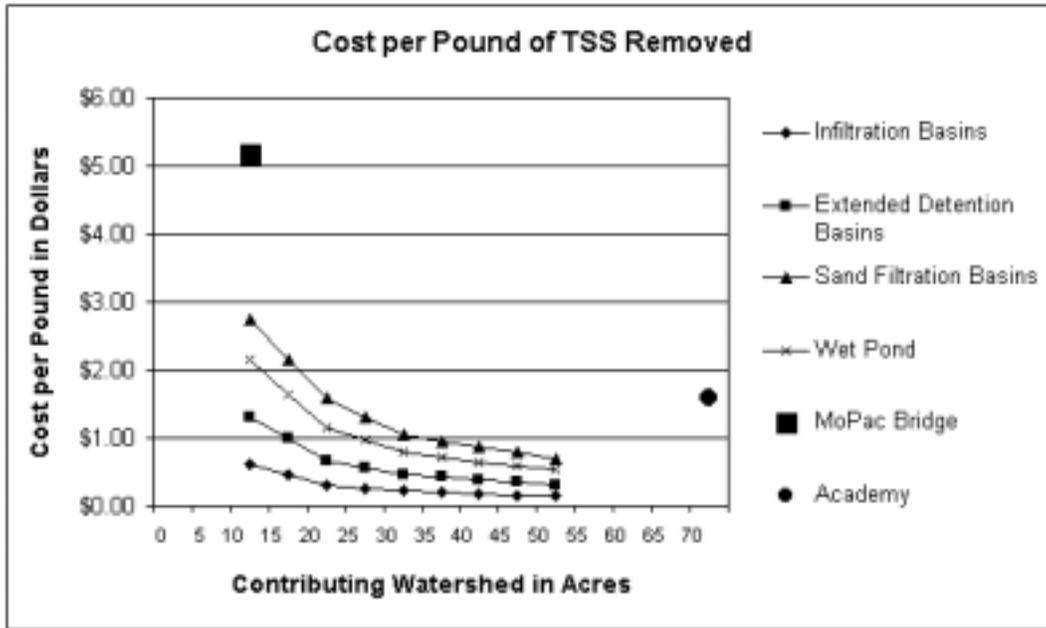
Fig. 3. All Earthen Structures: Cost to Performance by Watershed Size.
