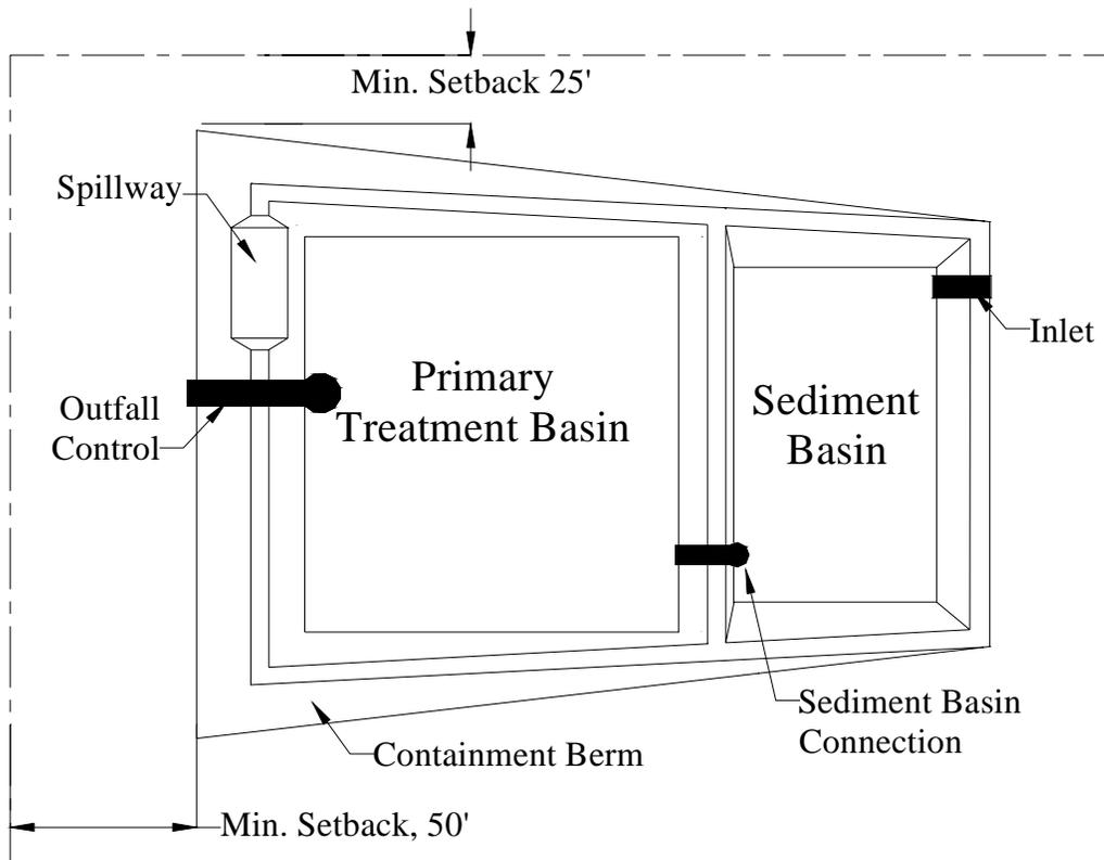
Fig. 1. Prototype Structure for Watersheds over 10 Acres.
