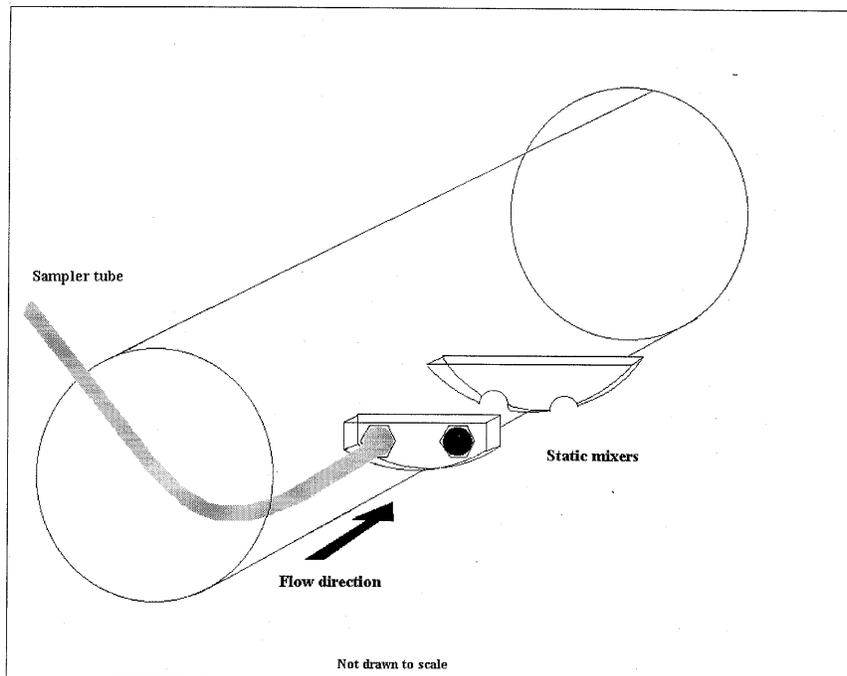
Fig. 3. Schematic diagram of a static mixer
