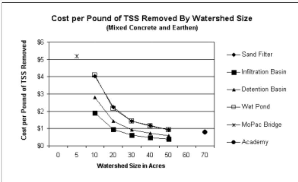
Fig. 4. Mixed Construction BMPs: Cost to Performance by Watershed
