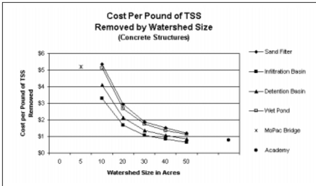
Fig. 2. All Concrete Structures: Cost to Performance by Watershed Size
